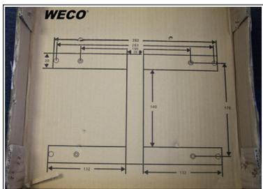
1. Drill the ceiling or cabin roof with the help of the drilling template printed inside the outer carton of the LED panel.
