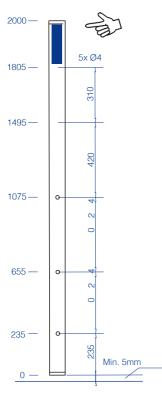
1.1) Securely fix the transmitter and receiver to the car/car doors through the fixing holes with the bolts provided, ensuring that the labels are pointing outwards.
