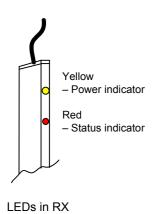
3.1) No LED in the receiver is lit. Cable is broken or not connected.
